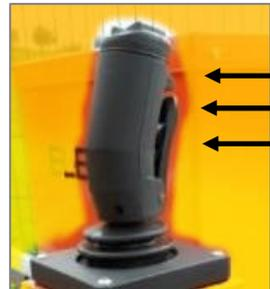
PRESS THE JOYSTICK DEAD MAN PRESENCE ENABLING CONTROL, then move the joystick forward/backward to lift/lower the cage
