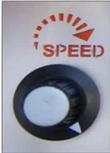
When the machine is in transport position (cage fully lowered), it is possible to regulate the transmission speed from the regulator. By turning the regulator anti-clockwise it is possible to lower the translation speed. On the other hand, by turning the regulator clockwise it is possible to increase the translation speed.
