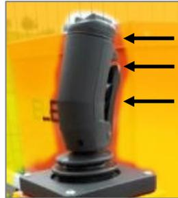
PRESS THE DEAD MAN BUTTON ON THE JOYSTICK, then move the joystick in the required direction.
