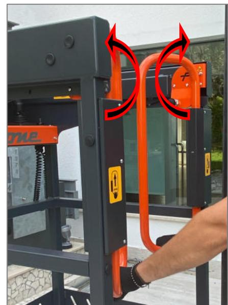
Access the cage by lifting the mobile doors slightly by pushing and rotating them inwards. Once the operator enters, he/she must close the gate, checking that the gate itself is locked properly, otherwise the machine will not enable any command.
