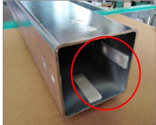
3. Insert eight new pads into the holes (2) made externally, on each side, at the end of the first extension;
