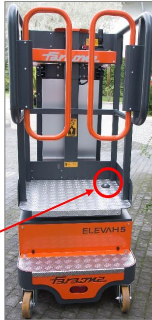
Place your foot on the switch, hold it down to actuate the joystick functions.
