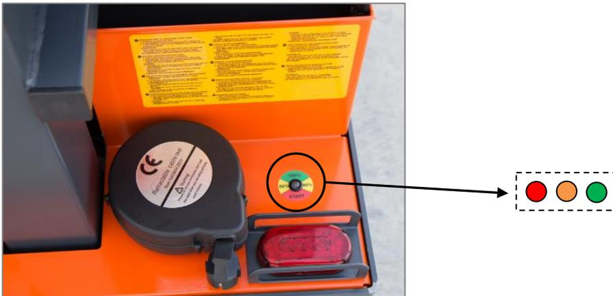
While recharging the battery, the **RED LED** indicates the beginning of the charging cycle. Charging stops automatically with no need for operator action, and is indicated by the **GREEN LED** on.
